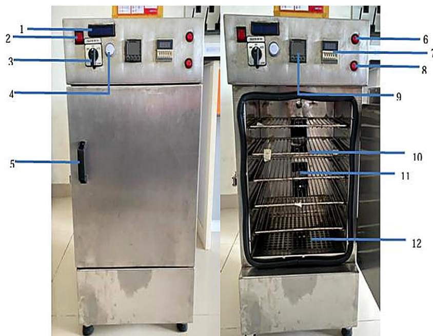
Figure 1. The dual-blower Biobriquette Tray Dryer used for the Drying Experiments
